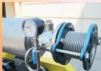
Inlet Flexible Connector (Stainless Steel 304) Vacuum Gauge Bypass Port
